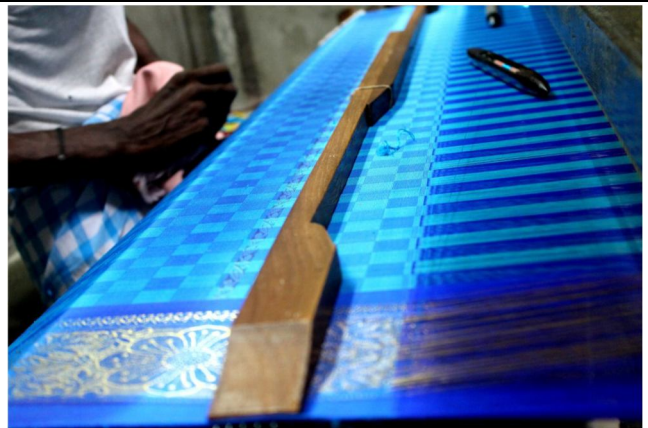
Figure 4: Throw shuttle to design patterns on saree
